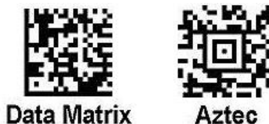
Obr. 10.12 2D kódy Data Matrix a Aztec [5]
